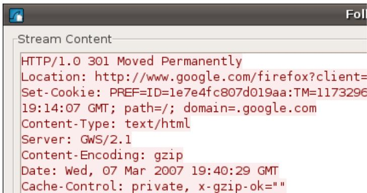
Right click a packet from the list (HTTP protocol, for example) and select "Follow TCP Stream" to link all packets that are sent between two computers and belong to a single protocol.
