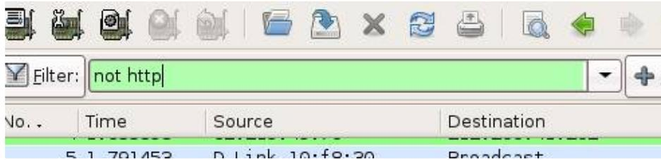
You can do that by right clicking a packet and selecting Apply as Filter, or by writing specific rules in the Filter textbox.
